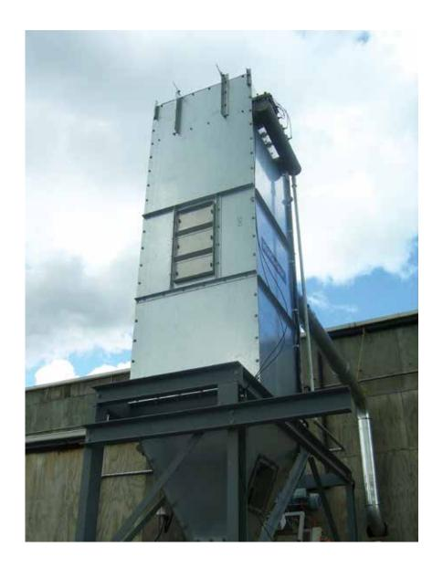
Our compact pulsejet dust collection systems provide an excellent solution for industrial applications where space is at a premium and where equipment needs to be relocatable.
