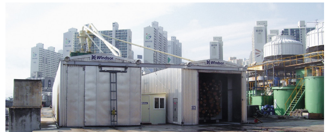
Windsor log conditioning chambers offer a simple effective system for softening logs.
